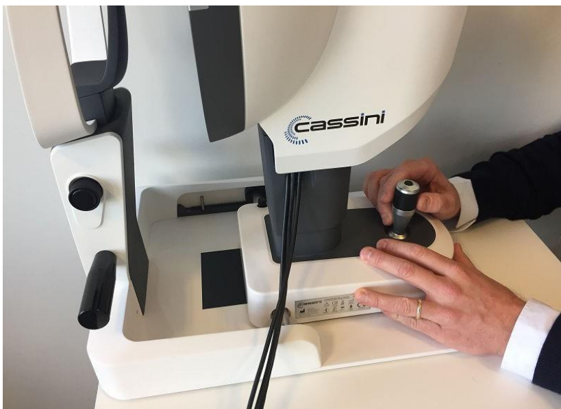
Figure 65: positioning Cassini (please use the non-joystick hand to increase control over the base if necessary)
