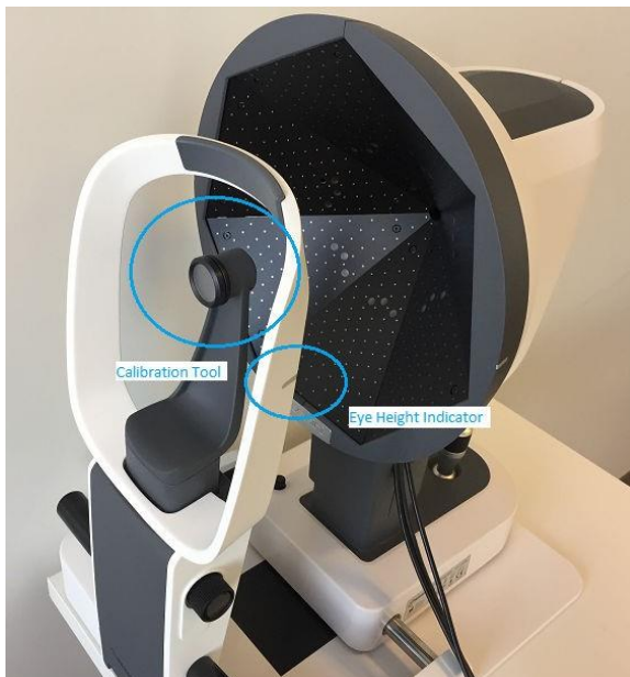
Figure 63: Calibration tool clamped in headrest (please note that the Cassini may look a bit different)
