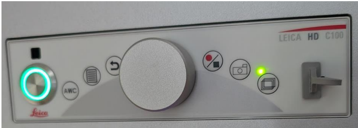
Figure 3. Leica HD C100 Control Module Front Panel Controls. Refer to the manual for a detailed explanation of the control functions.
