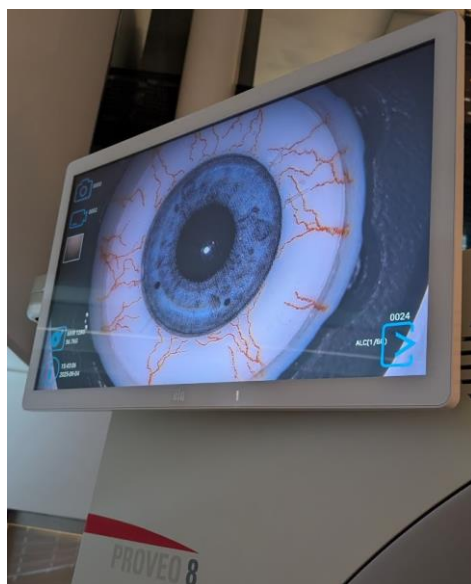
Figure 9. Microscope Camera feed on the microscope's own (control) monitor and/or existing display. Validated to match the Cassini's color and image orientation.
